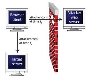
Figure 1: Firewall Circumvention Using Rebinding
