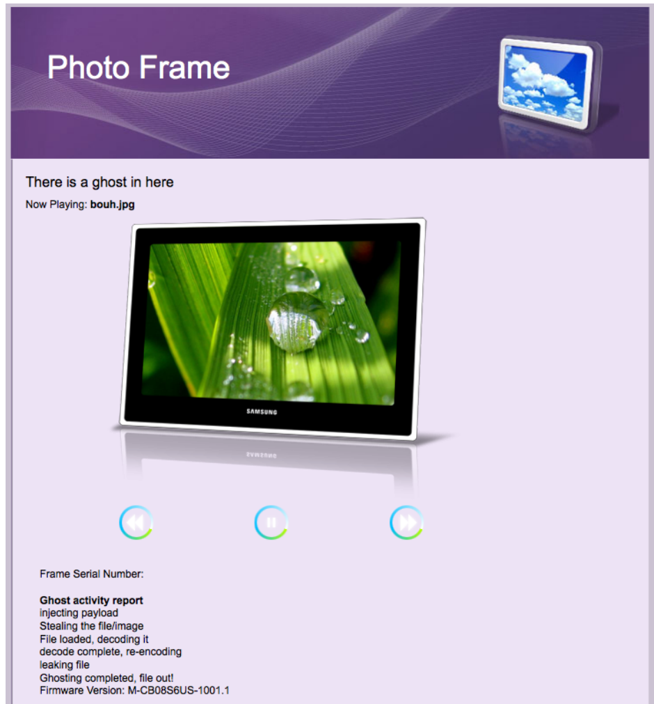
Figure 18: an RXCS attack in the Samsung photo frame that allows to steal photos.
