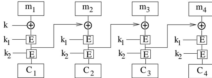
The secret key is a triple  $(k, k_1, k_2)$  where  $k$  is as long as  $E$ 's block size (64 bits for DES) and  $k_1, k_2$  are as long as  $E$ 's key size (56 bits for DES). For example, when  $E$  is DES the total key size is  $64+56+56 = 176$  bits.
