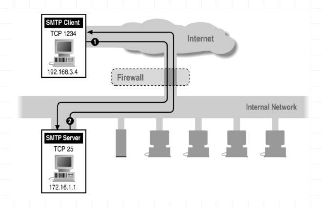
Can block external request to internal server based on port number
