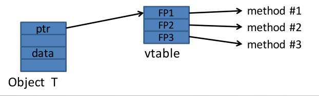
• Suppose vtable is on the heap next to a string object:
