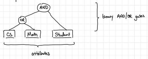
In a formula, every gate has fan-out 1 (each output of a gate. can only be used once)
